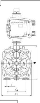
Height with controller fitted H2 + approx 246mm = 390mm
